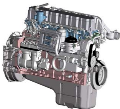
Figure 2: Engine cross-section view with DEUTZ-Common-Rail injection system (DCR©)
