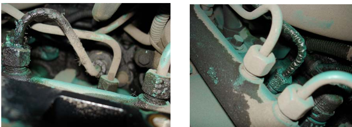
Figure 7: Damaged paintwork on the engine
