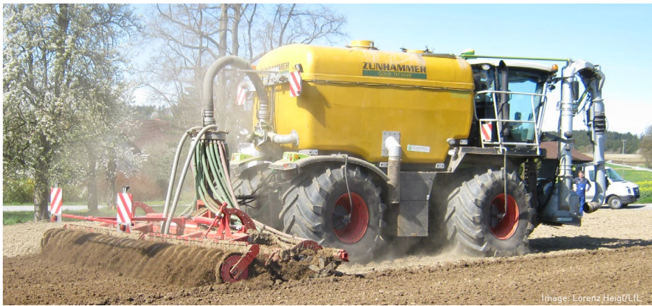
Ground-level application of manure
