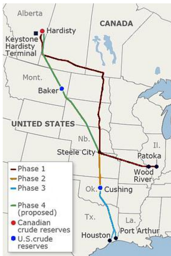
Figure 5 Keystone pipeline routes, including the yet to be approved phase 4 (keystone XL). Source: Wikimedia 2012
