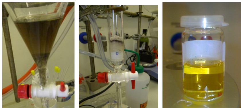
Fig. 2-8: Formation of a dark precipitate on the underside of the separating funnel (left); catalyst residue on silica gel (centre); catalyst-free biodiesel (right)
